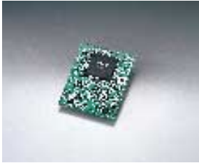
Image Processing Unit
